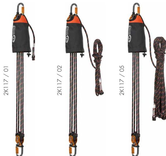
Auto-blocking rescue winch with 4x reduction factor, or 5x when used upside down, ideal for use in rescue manoeuvres. Developed to allow the lifting and the lowering of an injured operator or to tension a system.
