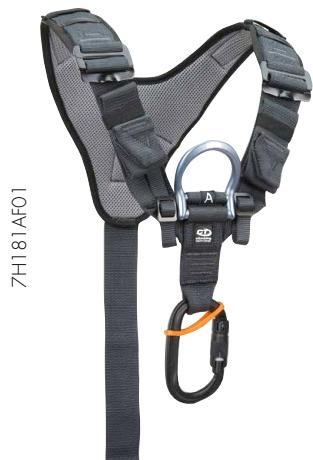
Detachable chest harness that, when connected to Xarrier sit harness, combines to form a full-body harness (EN 361 - EN 358 - EN 813) equipped with 5 attachment points. Contoured shoulder straps with shape optimized to avoid neck chafing.
