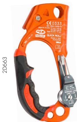
Innovative handled ascender, right or left-handed, with integrated pulley. Used in conjunction with a self-braking descender (e.g. Sparrow, Sparrow 200R) it allows for easier ascents along the work rope.
