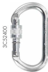
Zinc-plated steel oval connector with brass screw-up gate sleeve and traditional closure, suitable for harsh and dirty environments that could compromise the functioning of the Catch Free closure system.
