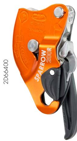
Self-braking descender for rope work, has been developed for high workloads. It allows the operator to lower themselves on the working line, to position themselves on it and to ascend the rope. It is ideal in the event of assisted lowering of two people with the device installed at the anchor (the operator lowers the rescuer and the person being rescued) or for simultaneous lowering of two people (rescuer lowers themselves with the injured person).
