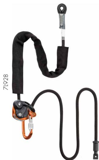
Multipurpose lanyard for work at height. Certified for use as an adjustable EN 358 work positioning lanyard, EN 795-B temporary anchor device and EN 795-C horizontal lifeline. The device is compliant with all requirements of the standard EN 12841-C for use as descender, except clauses 4.1.2 and 4.1.3 which have not been considered.
