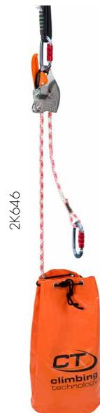
Rescue kit for work at height, developed for working loads up to 150 kg. It is made up of a fabric anchorage (Loop Ankor model - 120 cm), two oval connectors with triplex locking (Pillar TG model), a self-braking descender (Sparrow model), and a rope with end loops (Patron Plus 11 model).
