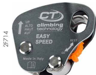
Fall arrest device designed for work at height and rope access. Compliant with the EN 353-2, EN 12841-A/B standards and RFU 11.075 requirements for use on inclined and horizontal surfaces over an edge ( $r \geq 0,5$  mm). It allows the safe ascent and descent along a vertical line, instantly locking in case of a fall.
