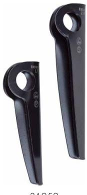
Angular hard steel piton. To be used on hard rock (granite, schist etc.) in large cracks. Excellent extraction strength due to its angular shape.
