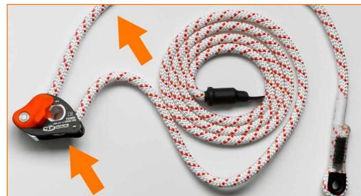
Regulator's connector and rope protection sheath missing.
