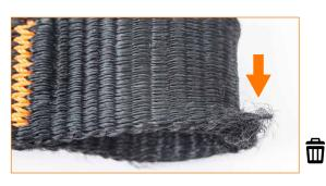
Elastic tape sling with end loop partially cut.
