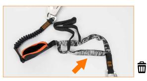
Energy absorber has been partially deployed.
