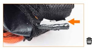
Missing labelling, label has been cut off.
