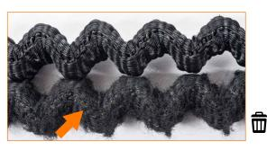
Elastic tape sling with clear evidence of wear (below), During the visual inspection the tape sling must be extended, so that hidden and potentially damaged parts can be examined.
