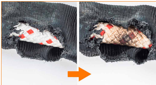
Clear burning on protection sheath. Important! Check the entire length of the rope: the damage on the sheath could be present on the rope as well.
