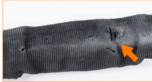
Clear burning on protection sheath. Important! Check the entire length of the rope: the damage on the sheath could be present on the rope as well.
