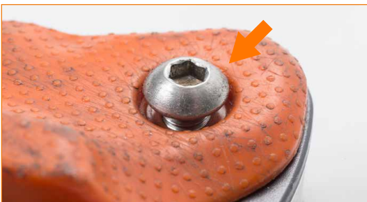
Regulator with loose screw. ⚠️ Apply low-strength thread-locking fluid and retighten until tight.
