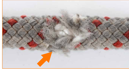
Rope with damaged sheath: the rope's core can be seen.
