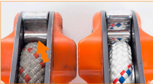
Regulator's cam very worn: see the difference between a new device (right) and one with a worn cam (left).
