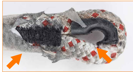
Termination loop damaged: thimble eye and heat-shrunk coating partially missing, stitching and rope worn and label illegible.
