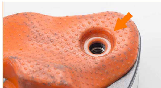
Regulator with missing screw. ⚠️ Replace with designated spare part. Apply low-strength thread-locking fluid and retighten until tight.
