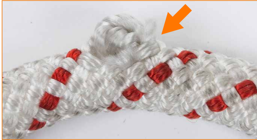
Rope core protruding.
