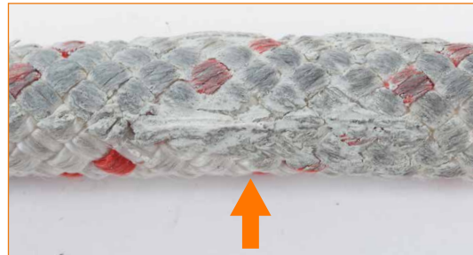
Rope very dirty with deposits of foreign substance.
