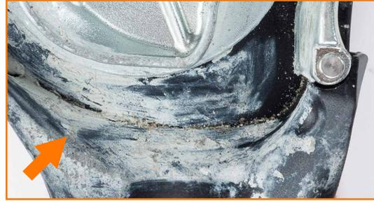
Locking cam does not automatically return to position and cam dirty with encrustations and deposits of foreign material.
