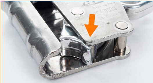
Deformed body that obstructs the opening of the locking lever.
