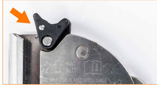
Safety lever that doesn't return autonomously into position.
