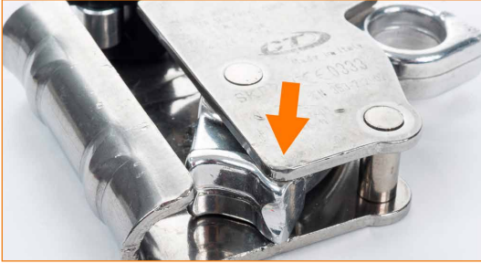
Bended locking cam.
