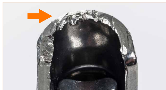
Body presenting cutting areas where the rope enters / exits: danger of damage of the rope!
