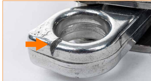
Locking lever with evident cracking signs.
