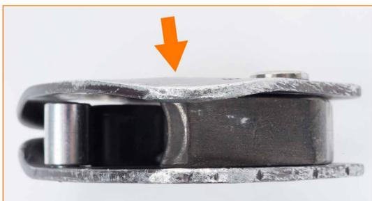
Fixed side plate bent and movement of locking cam impeded.
