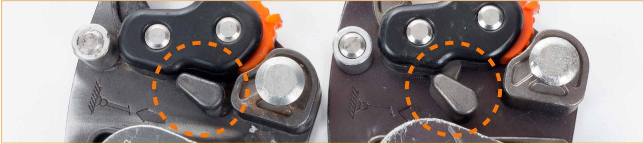
Resistance/drag when adjustment lever is moved: it should be able to move freely and immediately and automatically return to its position. On the left: an Easy Move with the adjustment lever stuck in an incorrect position: this defect prevents the device from working correctly. 🛠️ Clean with compressed air, wash with soap and water and lubricate with silicon-based oil spray . If the problem is not completely resolved, scrap the device.
