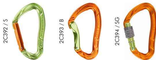
Light allow carabiner, hot forged with ample aperture, ideal for sport climbing and for intense use. Ergonomic shape with grip on the edge for perfect grip during use, with a double T ribbed profile for an excellent strength/weight ratio and elevated working loads.
